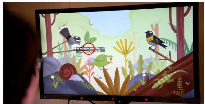
Figure 1: Setup on a regular desktop PC with a low-cost eye tracker. The viewer watches a video while gaze input is used to adapt the position of the captions. The gaze position is included for illustration purposes and is not visible in the application. 1
