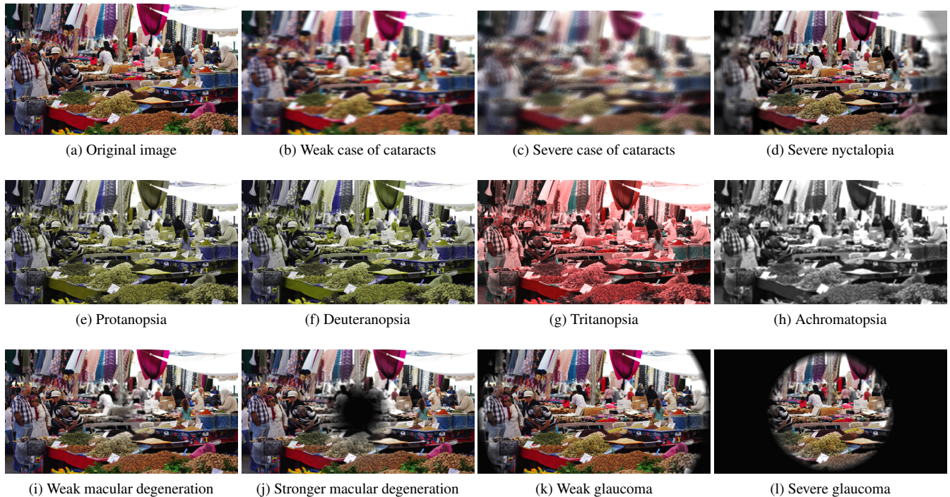
Figure 4: Simulation of non-refractive defects on an original unchanged image (a). Cataracts (b, c) showcase the first pass of our simulation. Various retinal maps in the last pass can simulate other vision disorders (d-l).
