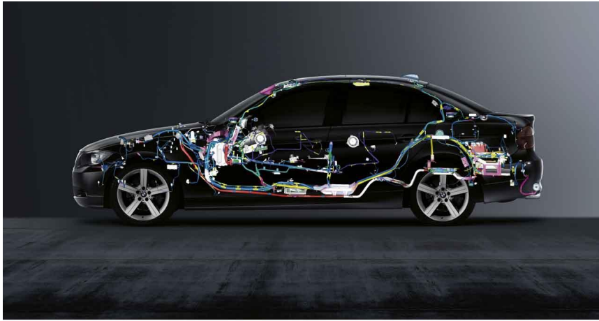
Figure 1.1: In-car communication network with ECUs, sensors and actuators.
