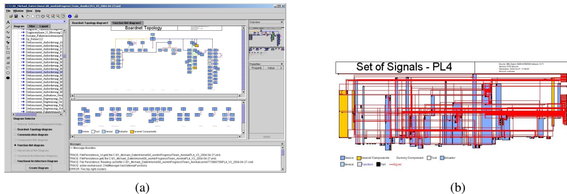
Figure 3.14: Screenshots of BNVis: (a) A Screenshot with a semi-automatically generated topology map; and (b) a signal diagram connecting several functional blocks automatically generated with BNVis.
