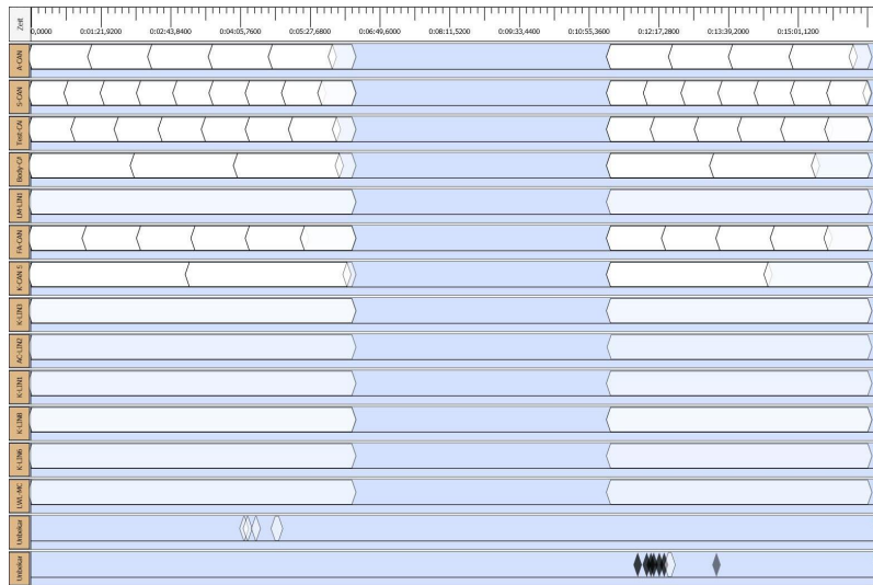
Figure 5.6: AutobahnVis ’ entirely zoomed-out Message View showing an overview over a 16-minute trace. The communication gap on all bus systems indicates a measuring hardware defect.
