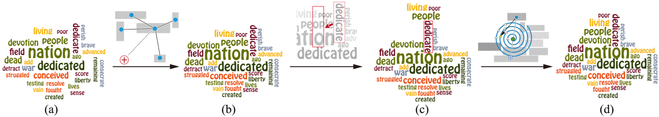
Fig. 2. Overview of our method: (a) given a Wordle, (b) we use our customized rigid body dynamics to move words close to each other; (c) if a word is moved, the forces update the words accordingly; (d) empty spaces are removed by using a local version of the Wordle algorithm.
