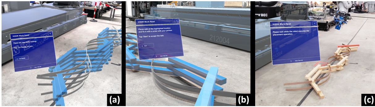
Figure 4: Three instruction interfaces shown to the user to provide task information. (a) initial prompt, (b) manual task execution prompt and (c) robotic task execution message.
