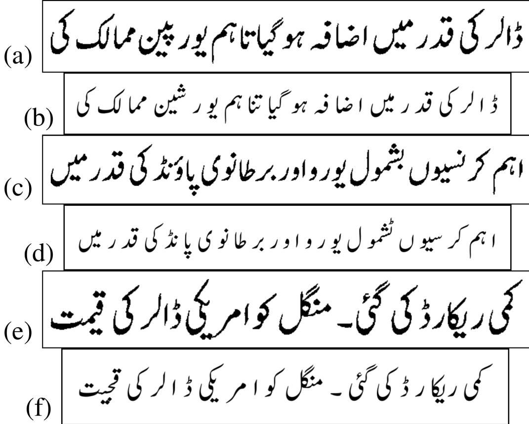
Figure 5.14: Input/output from the LSTM-based OCR illustrating capabilities and errors. (a), (c) and (e) represent the original images, whereas (b), (d) and (f) represent the output of LSTM network.
