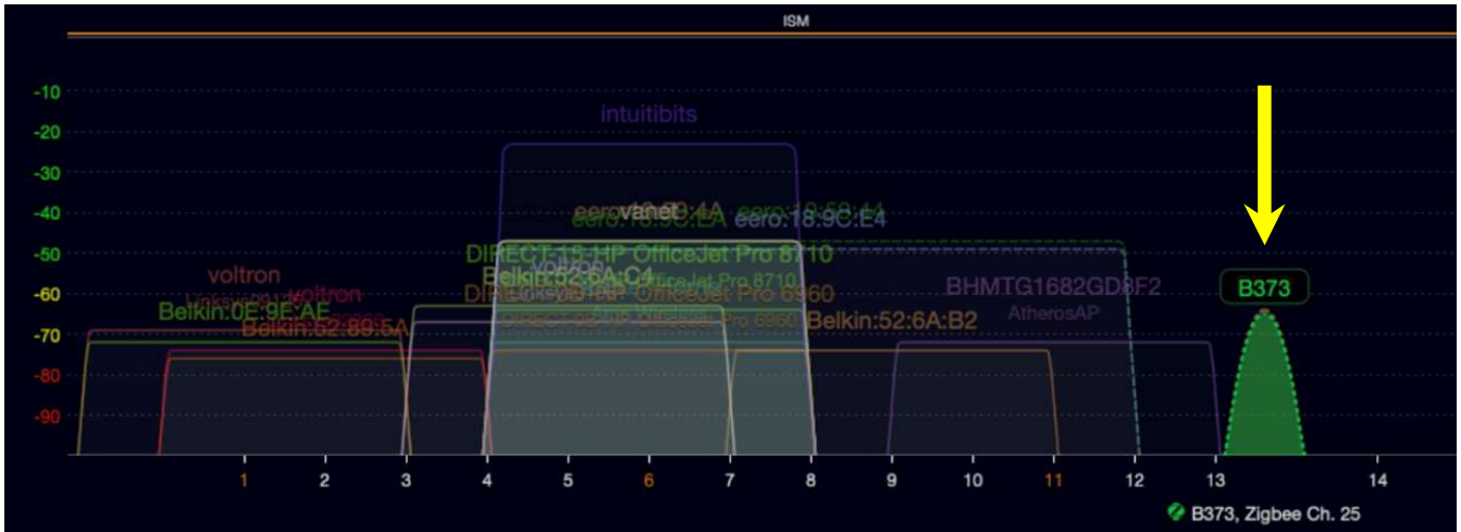
Figure 7-9 - Zigbee network overlaid on Wi-Fi networks
