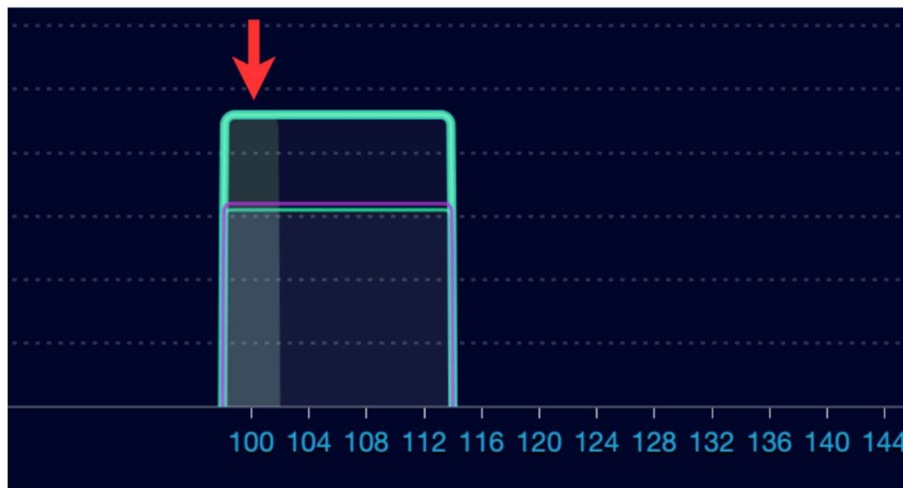
Figure 8-32 - Graphs Area : Spectrum 2.4/5 GHz panel indicating a primary channel (ch. 100)
