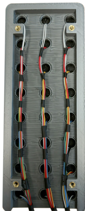
Figure 2: Example wiring of tactile array
