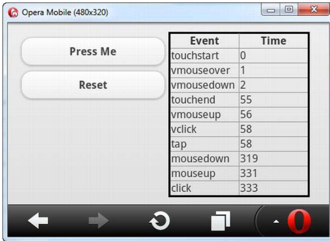
Figure 26-7. Adding the virtual events to the timing example
