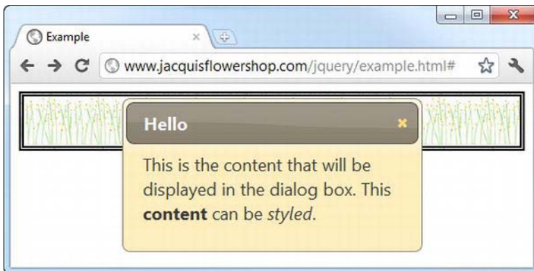
Figure 22-3. A dialog box with a custom title and no resize drag handle
