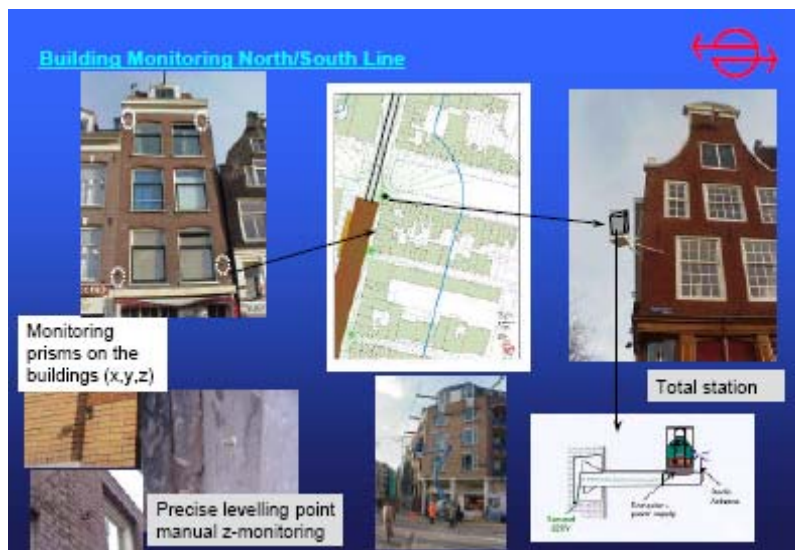
Figure 2.3: Monitoring system North/South metro line.
