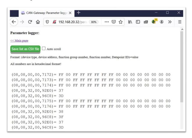
The parameters received are loaded each 5 seconds and added at the end of the list. The parameters can be exported to a CSV file.
