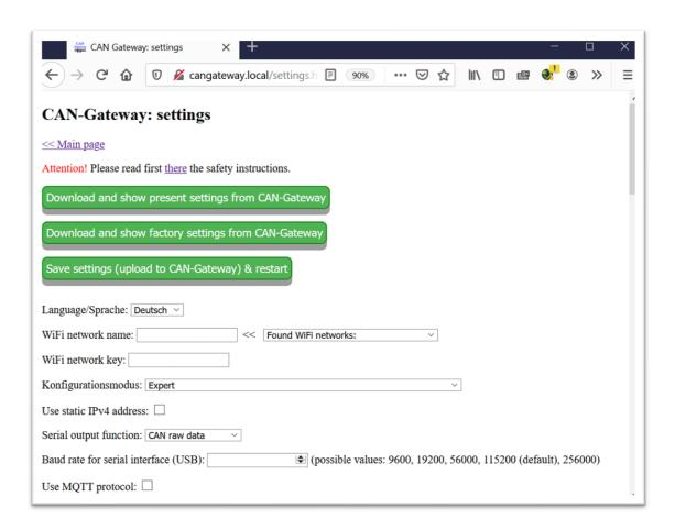
Before changing the settings, you should download and show the present settings of the CAN-Gateway. Then you can change them and click on "Save settings" to store changes on CAN-Gateway. After that the CAN-Gateway performs soft reset automatically.
