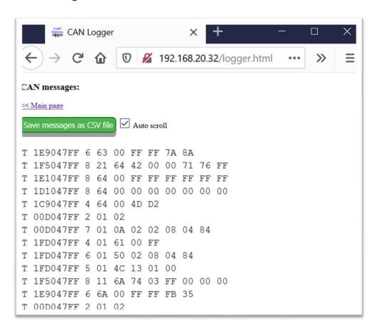
New messages received are loaded automatically each 5 seconds and shown at the end of the list. The messages can be exported to a CSV file. The first symbol "t" or "T" means a standard or extended CAN message frame. Then follow CAN-ID, DLC (data length) and 1 to 8 data bytes. Only messages containing can data are shown. RTR- and error-frames are ignored.
