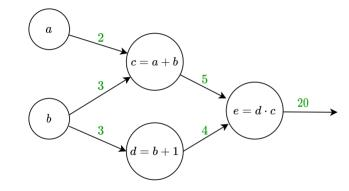
• We can assign the partial derivative to each edge of the graph.
