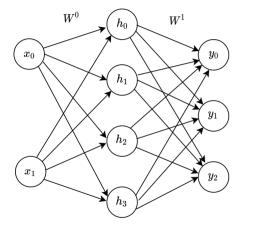
$egin{aligned} y &= \sigma(\mathcal{W}^1 \phi(\mathcal{W}^0 x)) \ h &= \phi(\mathcal{W}^0 x) \end{aligned}$
