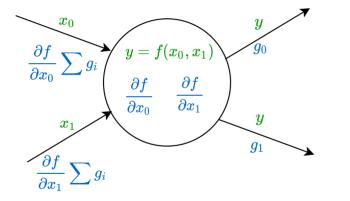
• Every node needs to implement a function and the partial derivatives of that function with respect to its inputs.
