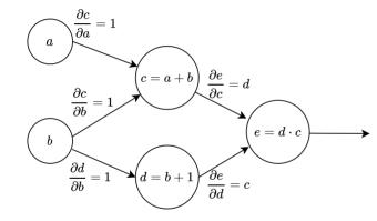
• After a forward pass through the network, we can assign a value to all of the partial derivatives by doing what is called a backward pass.
