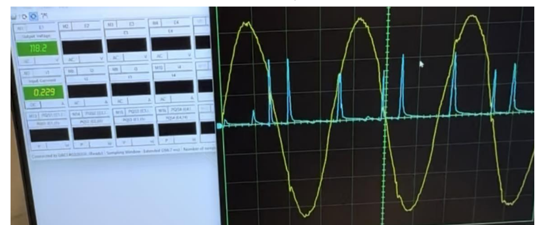
Figure 5. Outlet Receptacle Voltage (yellow), DC input current (blue)
