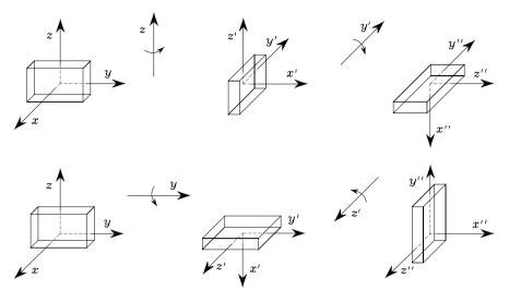
Fig. 2.6. Successive rotations of an object about axes of current frame
