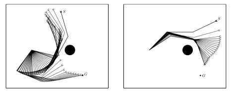
Fig. 12.16. Examples of motion planning via artificial potentials acting on control points for a planar 3R manipulator; *left*: planning is successful and leads to a collision-free motion between the start S and the goal G, *right*: a failure is reported because the manipulator is stuck at a force equilibrium
