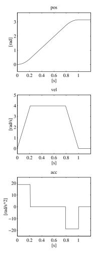
Fig. 4.3. Time history of position, velocity and acceleration with a trapezoidal velocity profile timing law
