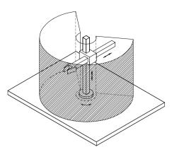
Fig. 1.4. Cylindrical manipulator and its workspace
