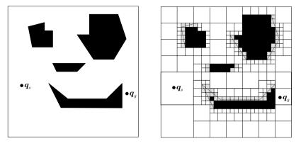
**Fig. 12.8.** An example of motion planning via approximate cell decomposition; *left*: the assigned problem, *right*: the solution as a free channel (*thick line*)
