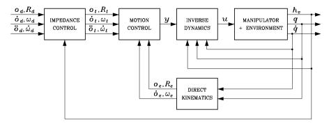
Fig. 9.5. Block scheme of admittance control
