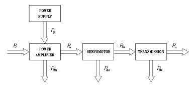
Fig. 5.1. Components of a joint actuating system
