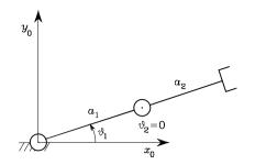
Fig. 3.3. Two-link planar arm at a boundary singularity
