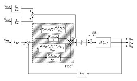
Fig. 8.17. Equivalent control scheme of  $PIDD^2$  type
