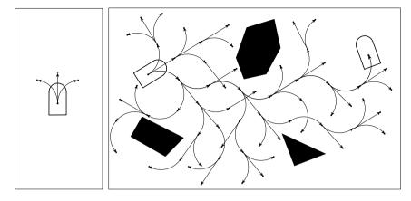
Fig. 12.11. RRT-based motion planning for a unicycle; *left*: a set of motion primitives, *right*: an example of RRT
