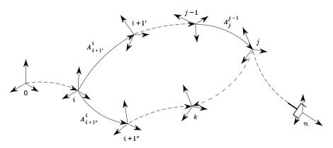
Fig. 2.18. Coordinate transformations in a closed kinematic chain
