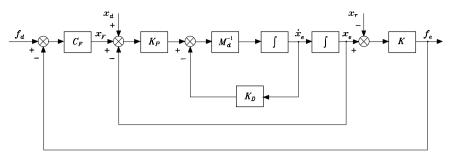
Fig. 9.8. Block scheme of parallel force/position control
