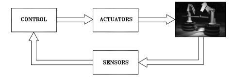
Fig. 1.1. Components of a robotic system
