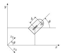
Fig. 11.3. Generalized coordinates for a unicycle
