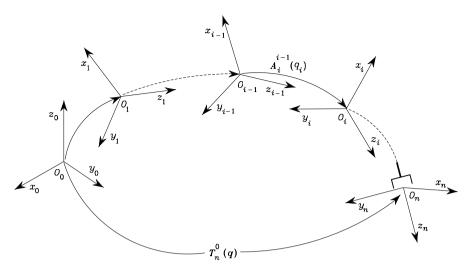
Fig. 2.15. Coordinate transformations in an open kinematic chain
