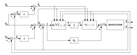
Fig. 8.26. Block scheme of joint space adaptive control
