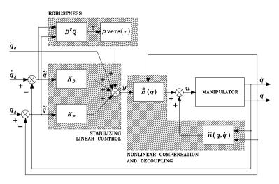
Fig. 8.23. Block scheme of joint space robust control
