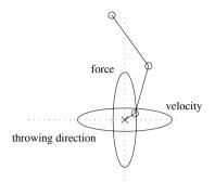
Fig. 3.27. Velocity and force manipulability ellipses for a 3-link planar arm in a typical configuration for a task of actuating force and velocity
