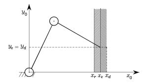
Fig. 9.1. Two-link planar arm in contact with an elastically compliant plane
