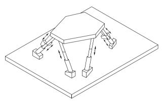
Fig. 1.9. Parallel manipulator
