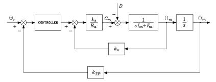
Fig. 5.9. General block scheme of electric drive control
