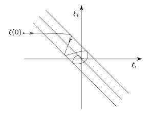
Fig. 8.25. Error trajectory with robust control and chattering elimination
