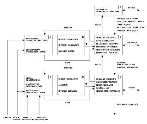
Fig. 6.2. Hierarchical levels of a functional architecture for industrial robots
