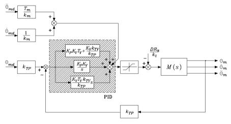
Fig. 8.16. Equivalent control scheme of PID type
