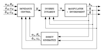
Fig. 9.2. Block scheme of impedance control
