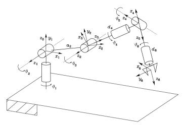
Fig. 2.26. Anthropomorphic arm with spherical wrist
