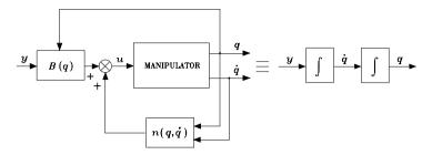
Fig. 8.21. Exact linearization performed by inverse dynamics control
