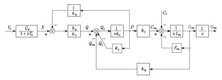
Fig. 5.6. Block scheme of a hydraulic drive
