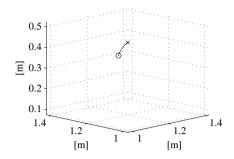
Fig. 10.29. Path of camera frame origin in Cartesian space with hybrid visual servoing
