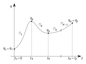
Fig. 4.4. Characterization of a trajectory on a given path obtained through interpolating polynomials
