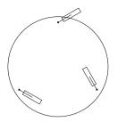
Fig. 1.17. An omnidirectional mobile robot with three independently driven caster wheels
