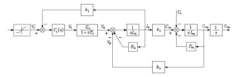
Fig. 5.2. Block scheme of an electric drive
