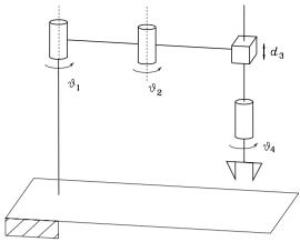
Fig. 2.36. SCARA manipulator
