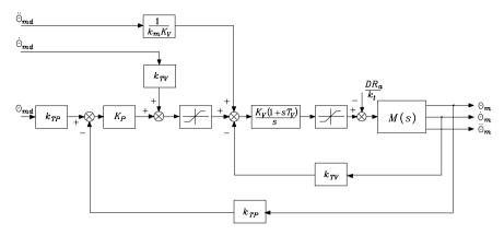
Fig. 8.13. Block scheme of position and velocity feedback control with decentralized feedforward compensation
