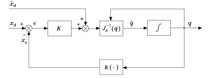
Fig. 3.11. Inverse kinematics algorithm with Jacobian inverse
