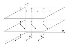
Fig. 11.2. A local representation of the configuration space for the rolling disk with an example manoeuvre that transfers the configuration from  $q_i$  to  $q_f$  (dashed line)
