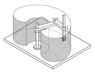
Fig. 1.6. SCARA manipulator and its workspace
