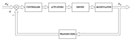
Fig. 8.2. General scheme of operational space control
