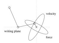
Fig. 3.26. Velocity and force manipulability ellipses for a 3-link planar arm in a typical configuration for a task of controlling force and velocity
