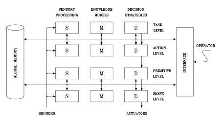
Fig. 6.1. Reference model for a control system functional architecture
