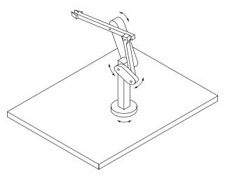
Fig. 1.8. Manipulator with parallelogram
