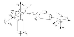
Fig. 2.24. Spherical wrist
