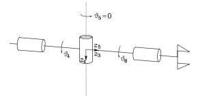
Fig. 3.4. Spherical wrist at a singularity
