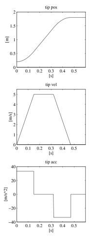
Fig. 7.9. Time history of tip position, velocity and acceleration with a straight line tip trajectory along the horizontal axis
