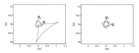
Fig. 11.10. Planning a pure reorientation manoeuvre via the chained form; *left*: with the coordinate transformation (11.23), *right*: with the coordinate transformation (11.52)
