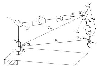
Fig. 2.32. Manipulator with spherical wrist
