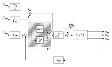
Fig. 8.15. Equivalent control scheme of PI type
