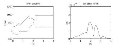
Fig. 8.39. Time history of the joint torques and of the norm of tip position error for the *fast* trajectory with control scheme L
