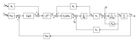
Fig. 8.18. Control scheme with current-controlled drive and current feedforward action
