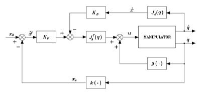
Fig. 8.29. Block scheme of operational space PD control with gravity compensation
