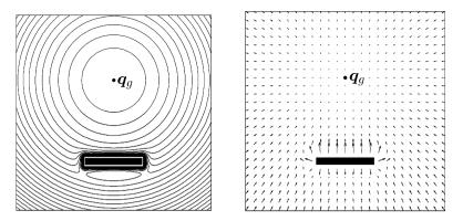
**Fig. 12.14.** The total potential in  $C = \mathbb{R}^2$  obtained by superposition of a hyperboloidic attractive potential and a repulsive potential for a rectangular *C*-obstacle: *left*: the equipotential contours, *right*: the resulting force field
