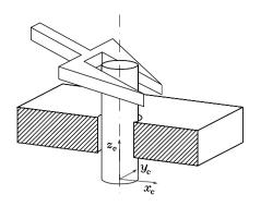
Fig. 9.13. Insertion of a cylindrical peg in a hole
