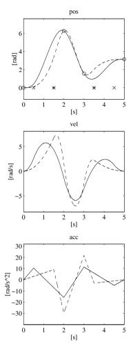
Fig. 4.7. Time history of position, velocity and acceleration with a timing law of cubic splines for two different pairs of virtual points
