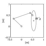
Fig. 7.15. Effect of gravity on the dynamic manipulability ellipsoid for a three-link planar arm
