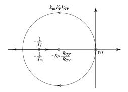
Fig. 8.8. Root locus for the position and velocity feedback control scheme
