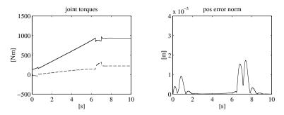
Fig. 8.42. Time history of the joint torques and of the norm of tip position error for the *slow* trajectory with control scheme  $\mathbf{E}$
