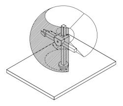
Fig. 1.5. Spherical manipulator and its workspace
