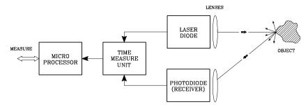
Fig. 5.20. Time-of-flight laser sensor operating principle
