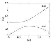
Fig. 3.24. Minimum and maximum singular values of J for a two-link planar arm as a function of the arm posture
