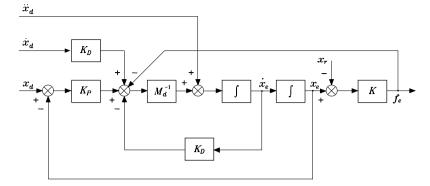
Fig. 9.3. Equivalent block scheme of a manipulator in contact with an elastic environment under impedance control
