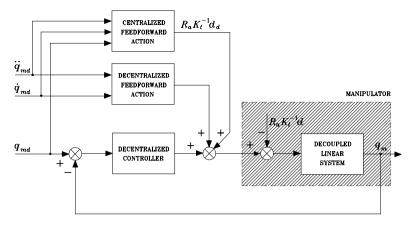
Fig. 8.19. Block scheme of computed torque feedforward control
