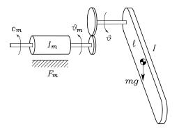
Fig. 5.8. Pendulum actuated via mechanical gear
