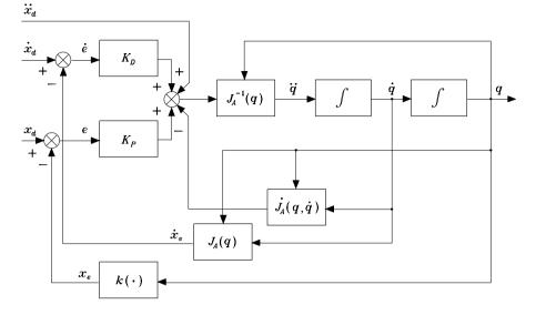
Fig. 3.14. Block scheme of the second-order inverse kinematics algorithm with Jacobian inverse
