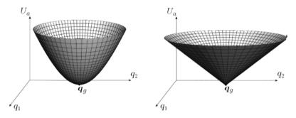
Fig. 12.12. The shape of the paraboloidal attractive potential  $U_{a1}$  (*left*) and of the conical attractive potential  $U_{a2}$  (*right*) in the case  $C = \mathbb{R}^2$ , for  $k_a = 1$
