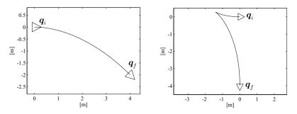
Fig. 11.8. Two parking manoeuvres planned via the chained form
