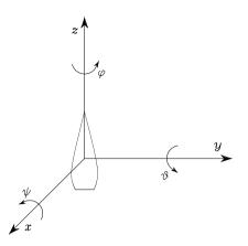
Fig. 2.9. Representation of Roll–Pitch–Yaw angles
