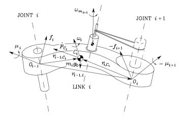
Fig. 7.13. Characterization of Link i for Newton–Euler formulation
