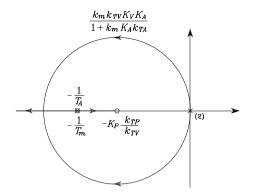
Fig. 8.10. Root locus for the position, velocity and acceleration feedback control scheme  $% \mathcal{F}_{\mathrm{rel}}^{(1)}(\mathcal{F}_{\mathrm{rel}})$
