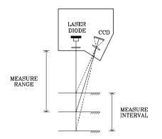
Fig. 5.21. Triangulation laser sensor operating principle
