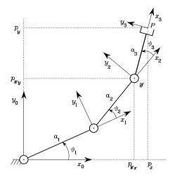
Fig. 2.20. Three-link planar arm
