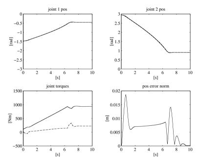
Fig. 8.43. Time history of the joint positions and torques and of the norm of tip position error for the *slow* trajectory with control scheme  $\mathbf{F}$
