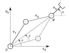
Fig. 2.31. Admissible postures for a two-link planar arm
