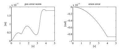
Fig. 3.15. Time history of the norm of end-effector position error and orientation error with the open-loop inverse Jacobian algorithm
