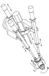
Fig. 1.10. Hybrid parallel-serial manipulator
