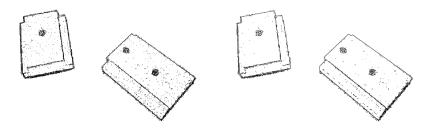
**Fig. 10.3.** Contours of image of Fig. 10.1 obtained using Roberts (*left*) and Sobel (*right*) operators
