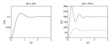
Fig. 9.4. Time history of the tip position along vertical direction and of the contact force along horizontal direction with impedance control scheme for environments of different compliance
