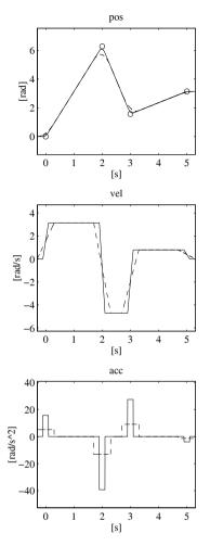
Fig. 4.9. Time history of position, velocity and acceleration with a timing law of interpolating linear polynomials with parabolic blends
