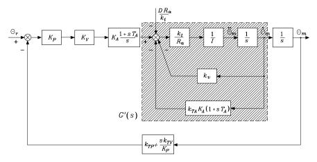
Fig. 8.9. Block scheme of position, velocity and acceleration feedback control
