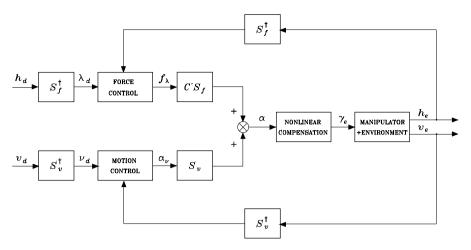
Fig. 9.15. Block scheme of a hybrid force/motion control for a compliant environment
