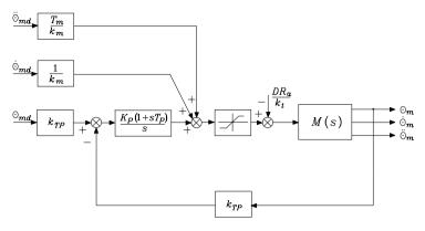
Fig. 8.12. Block scheme of position feedback control with decentralized feedforward compensation
