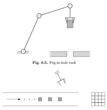
Fig. 6.6. Palletizing task of objects available on a conveyor
