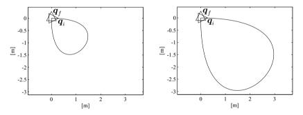
Fig. 11.7. Planning a pure reorientation manoeuvre via cubic Cartesian polynomials; *left*: with k = 10, *right*: with k = 20
