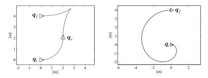
**Fig. 11.9.** Planning a parallel parking manoeuvre via the chained form; *left*: adding a via point  $q_v$ , *right*: letting  $\theta_f = \theta_i + 2\pi$
