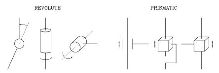
Fig. 2.12. Conventional representations of joints
