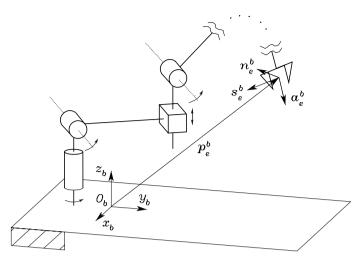
Fig. 2.13. Description of the position and orientation of the end-effector frame
