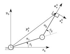
Fig. 2.14. Two-link planar arm
