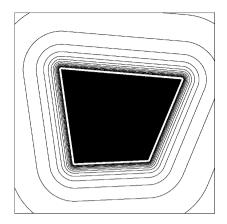
Fig. 12.13. The equipotential contours of the repulsive potential  $U_r$  in the range of influence of a polygonal C-obstacle in  $C = \mathbb{R}^2$ , for  $k_r = 1$  and  $\gamma = 2$
