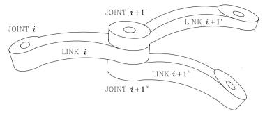
Fig. 2.17. Connection of a single link in the chain with two links
