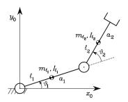
Fig. 7.4. Two-link planar arm
