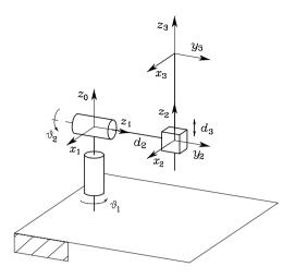
Fig. 2.22. Spherical arm
