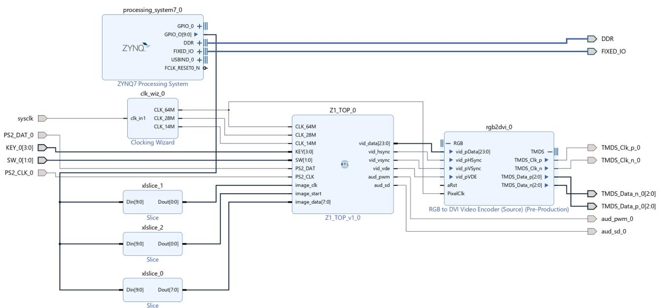
The bulk of the system is inside the RTL module Z1\_TOP\_0 (middle). The ZYNQ7 Processing System (top-left) is the CPU in the SoC (PS in Xilinx terms). The ARM CPU is connected to the Z1\_TOP\_0 module with GPIO pins, to
