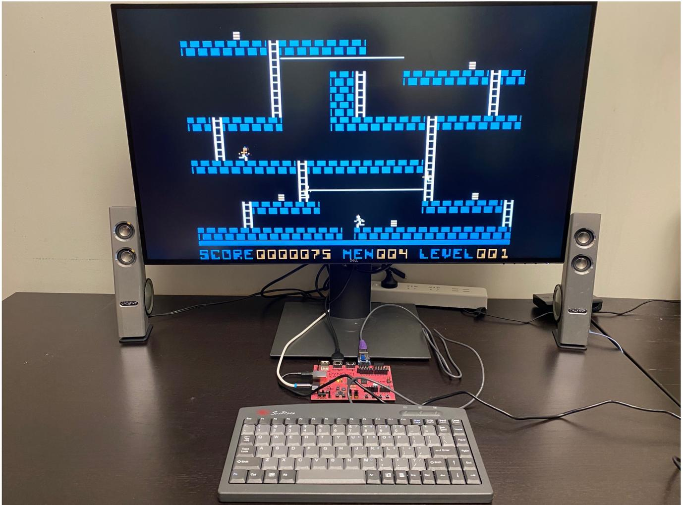
The main chip of PYNQ-Z1 is Xilinx ZYNQ XC7Z020-1CLG400C, a so-called FPGA SoC (System-on-Chip). In addition to FPGA logic, it also contains a dual-core ARM A9 CPU, hence the SoC name.
